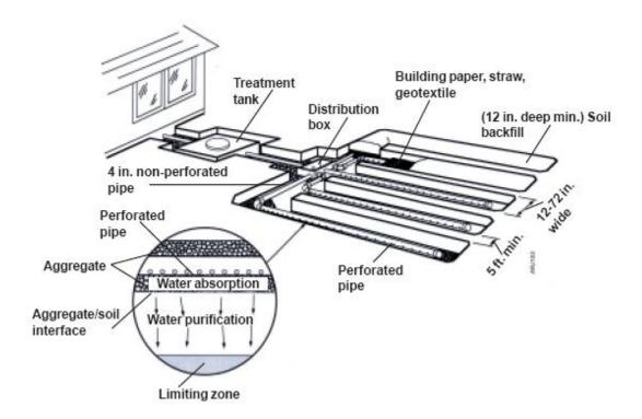
**Diagram of Typical Drainfield Showing Underground Trenches**
