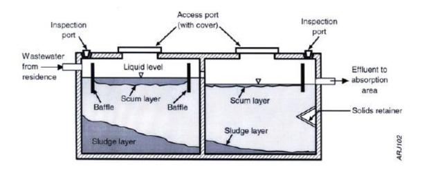
Cross Section of a typical Two Compartment Septic Tank
